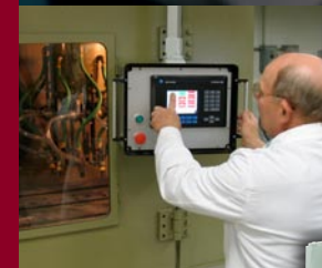
Automated ZERO blast cabinet with "touch-screen" operator interface
